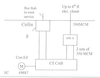
This existing installation provides a 500 MCM to  $6^{th}$  floor for Owner's use. The following must be done:
